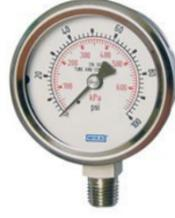
A pressure gauge reads the system pressure at the point where the gauge is at in the system. It is not reading pump discharge pressure unless it is mounted directly at the pump discharge.
