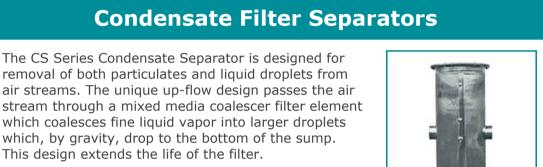
which coalesces fine liquid vapor into larger droplets which, by gravity, drop to the bottom of the sump.
