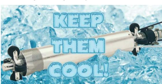
The EPG SurePump intake screen is located below the motor and the sealed top ensures that the liquid is drawn only from the bottom and over the entire motor. Wheels improve mobility and suspend the pump above sediment on the floor of the riser pipe.
