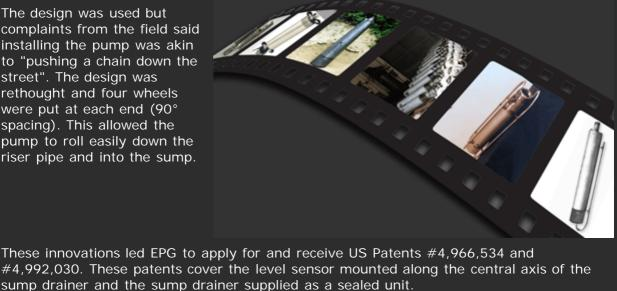
The sump drainer design is simple, yet effective. Since the unit is sealed, all the leachate is drawn through the bottom intake screen, past the motor and into the pump's intake. The
