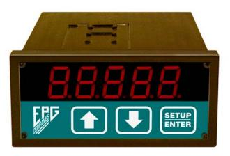
The meter has a nominal display rate of 2.5 updates per second, a response time of 500 ms per input step, will store the highest and lowest readings in meter memory until cleared, and has a built-in 24VDC power supply for 4-20 mA sensors. The meter is also equipped with transducer overload and short-circuit protection.
