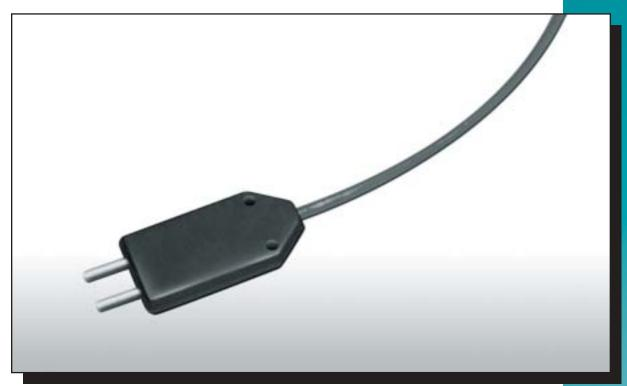
EPG Leak Detection Sensors are designed to be used in landfill recirculation and bioreactor systems to detect leakage. Conductance is made from probe to probe through the presence of liquid. Typically, the sensor sends a signal to an intrinsically safe relay which can be used to annunciate an alarm condition or shut equipment down. The control circuit has an energy potential so low that it is incapable of causing ignition of flammable or combustible materials.
