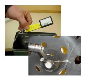
Data Logger with Thermocouple and Flame Pilot Tube
