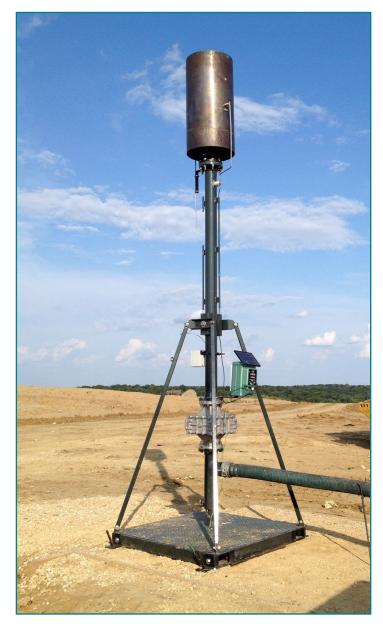
*Data Station to monitor and record flow, temperature and gas quality is also available.*
