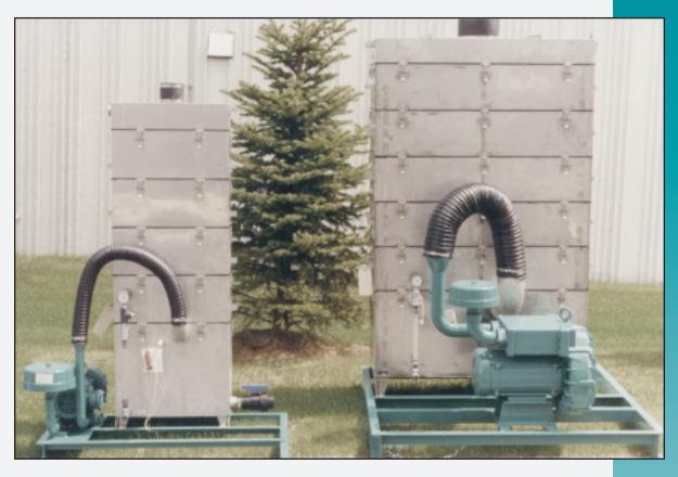
EPG offers low-profile tray air strippers for removal of volatile organic compounds (VOCs) from liquids. They are used effectively for treatment of contaminated groundwater and process water.
