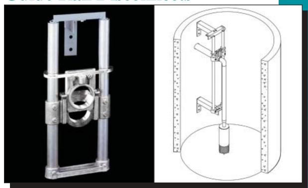
EPG's Heavy Duty Guide Rail Disconnects are constructed from high quality materials for long life and durability. They are designed for use in any basin/pump combination with standard stainless steel guide rails for easy pump connection and disconnection. A unique feature in the guide rings allows the removable half of the disconnect to slide off the guide rails with out removing the top.
