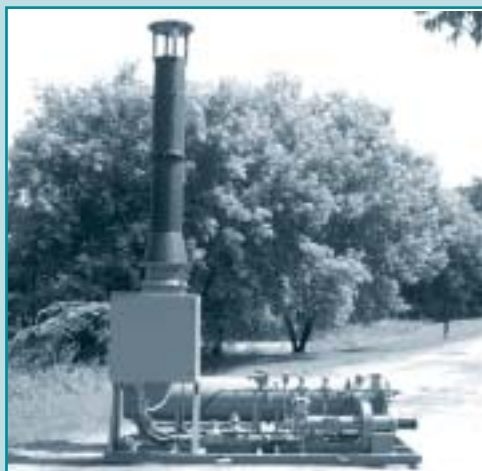
Skid Mounted Thermal Oxidizer
