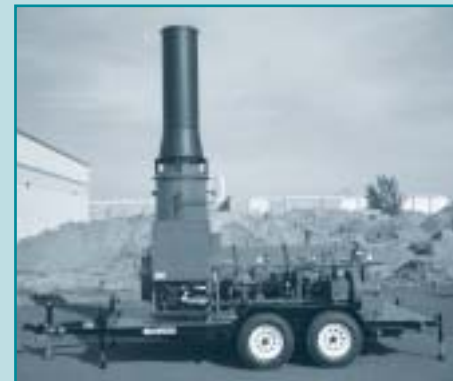
Trailer Mounted Thermal Oxidizer
