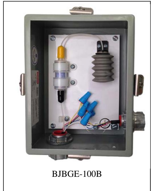
Inside of the box is a desiccant dryer and equalizing bellows to protect the back side of the sensor from moisture and landfill gas. In addition, water-proof wire connectors are provided to prevent corrosion.
