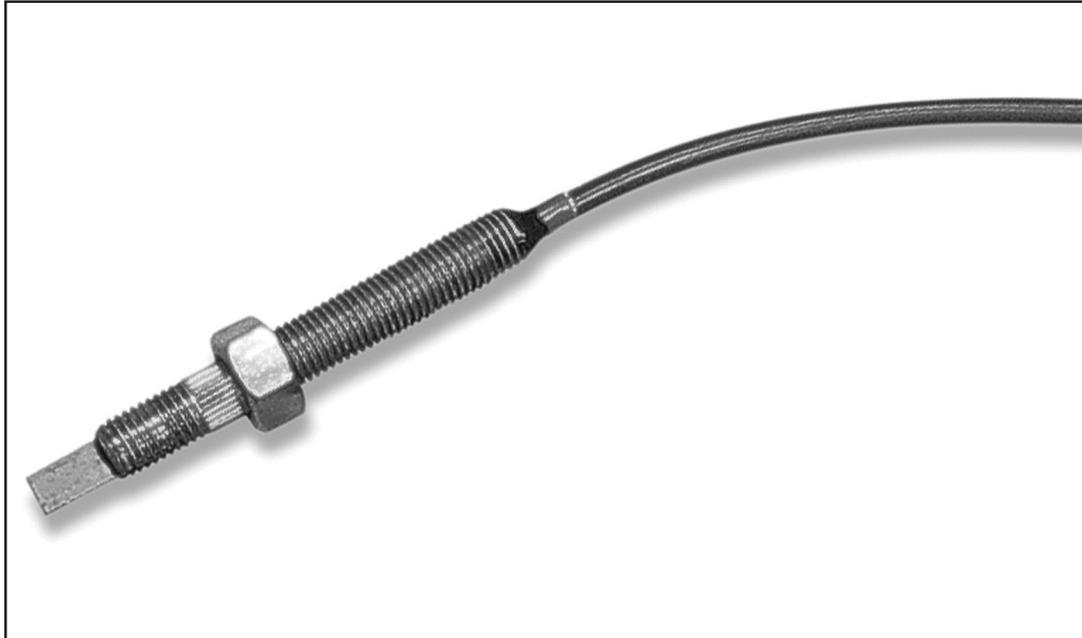
EPG Temperature Switches are used in EPG pump motors to sense over temperature conditions. If the temperature of the motor reaches a critical pre-determined limit, the normally closed temperature switch will open, sending a motor shut down and/or operator alert signal. When the motor temperature falls below the critical limit, the temperature switch will close and reset itself.
